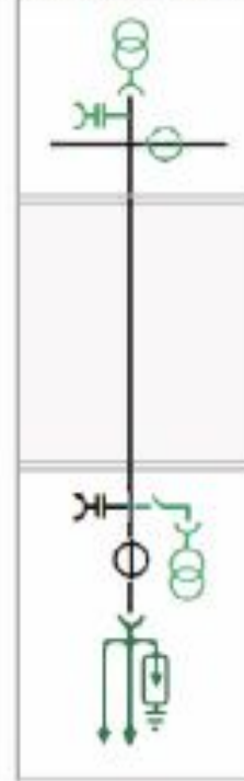
Direct connection panel
