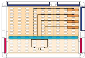
Vertical circuit-breaker with rear terminals with rear intermediate upright*
